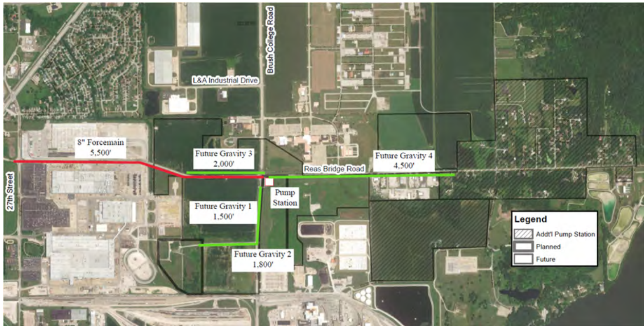
Figure 2. Preliminary Pump Station and Sewer Layout
