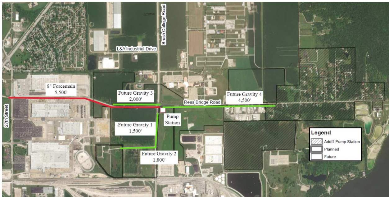
Figure 2 – Preliminary Pump Station and Sewer layout
