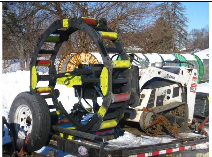
The spiral winding machine that will be inserted into the sewer.
