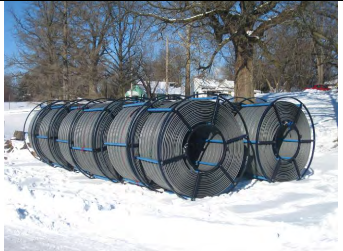
Spools of the steel reinforced PVC lining panels.
