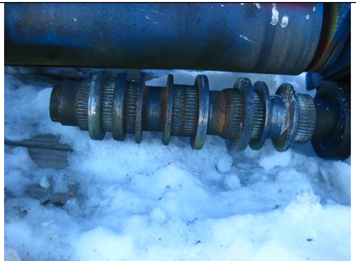
Grooved head that will snap the liner in place.
