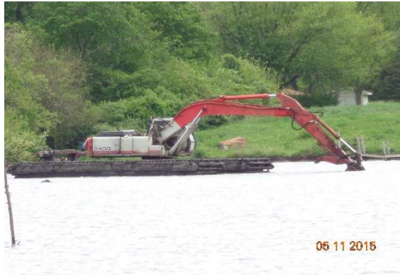
Swamp excavator at work digging up stumps in Big Creek Basin.
