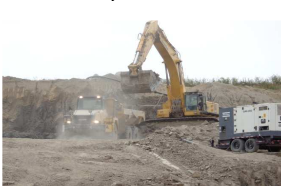
Excavator with 8 yard bucket loading a 40 ton dump truck.
