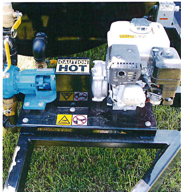
On-board Pumping System
