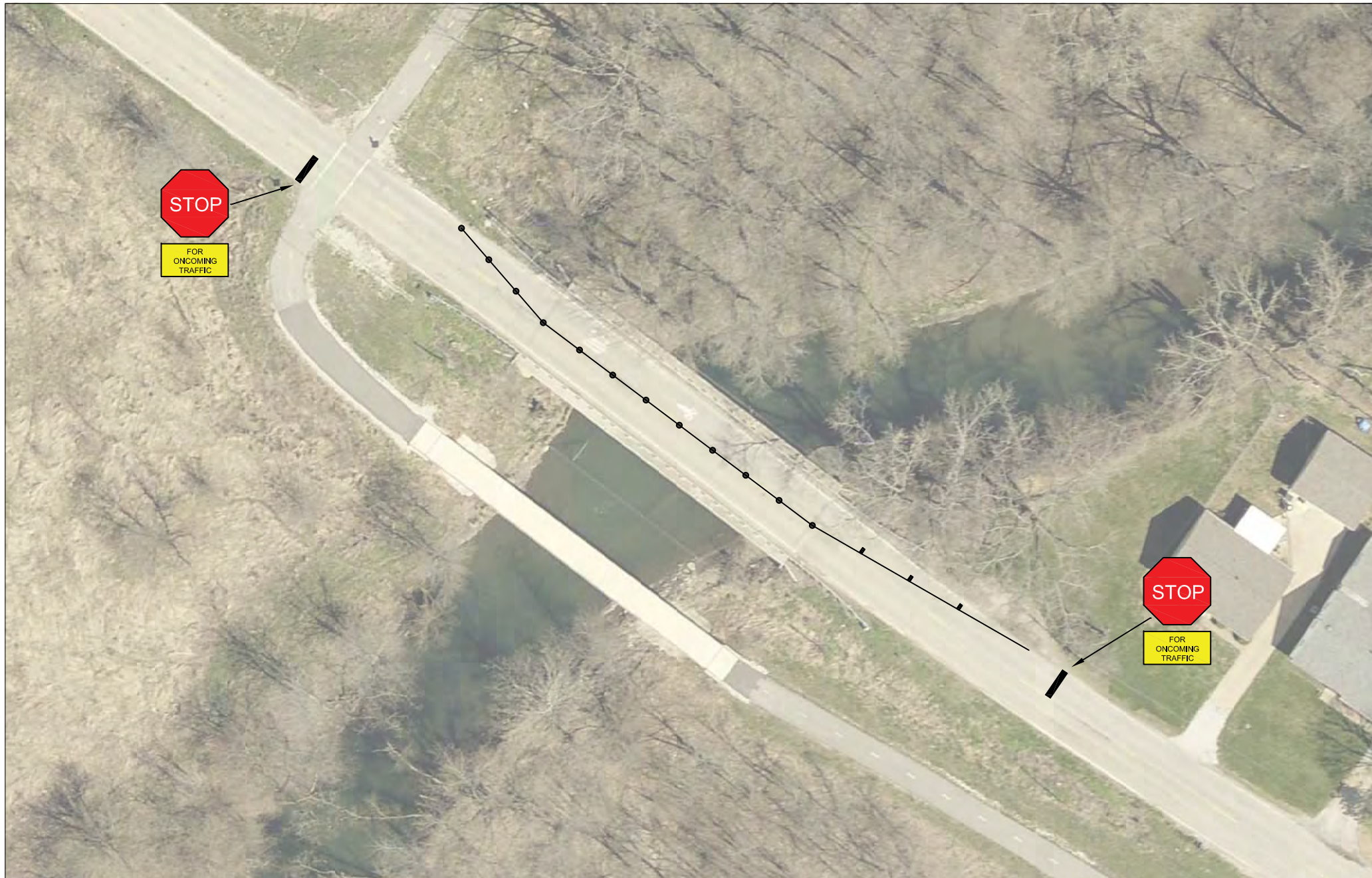
Figure 1 Traffic Control for Center St. Bridge as a One-Lane Bridge
